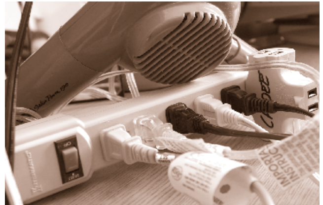
Copy of Overloaded Power Strip Courtesy of Underwriters Laboratories
