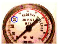
If used for cleaning purposes, must be maintained less than 30 psi: 29 CFR 1910.242(b)
